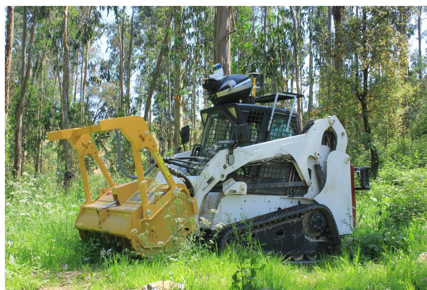
Figure 3: Heavy-duty UGV used in the SEMFIRE and SafeForest projects in a forest environment.
