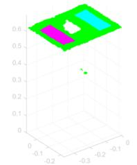
Figure 1 - Point Cloud with segmented bands. The left band is colored in magenta and the right band is colored in cyan.
