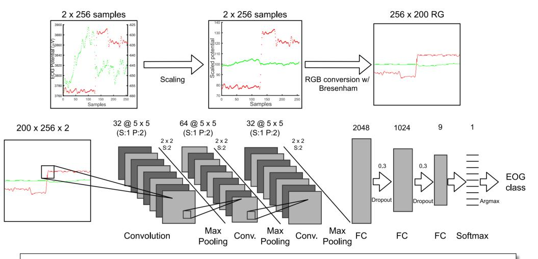
Scaling, conversion and CNN classification of EOG signals take place before the class is inputted to the EUDN, the precursor to the RL pipeline
